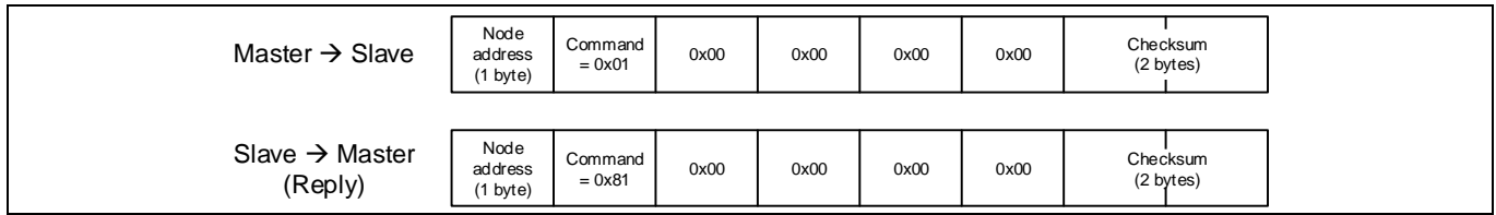
Figure 35 Clear fault command
